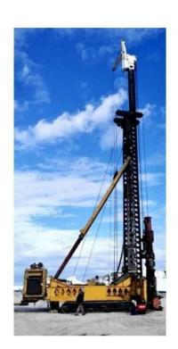
This rig comes with a special frame that can be mounted on the rear side on which you can place a hydraulic power pack when using this rig for drilling or for cast in situ piles. If no power pack is used we recommend to put a steel or concrete weight on the frame to act as extra counterweight. Recommended weight 6.000 kg.
